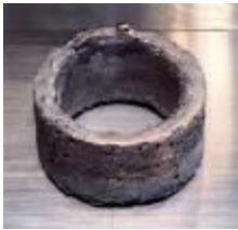
A 99.96% pure ring of Plutonium
