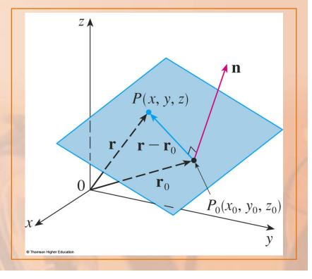
The normal vector **n** is orthogonal to every vector in the given plane. In particular, **n** is orthogonal to  $\mathbf{r} - \mathbf{r}_0$ .
