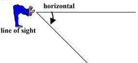
The Angle of Depression is the angle from the horizontal to the line of sight. (i.e. you are looking downwards at the
