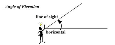
The Angle of Elevation is the angle from the horizontal to your line of sight. (i.e. you are looking upwards at the object)
